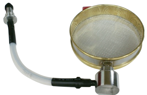
Coupling of adapter, test sieve & transducer
